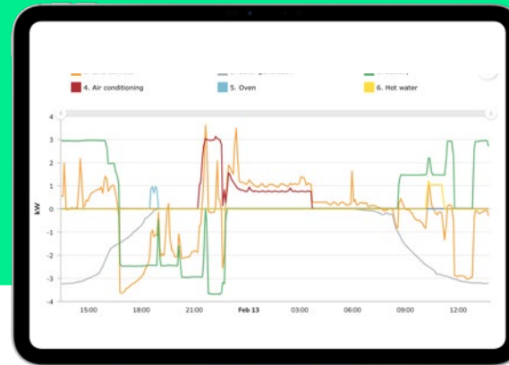
WattWatchers: Monitoring household energy usage and solar generation (data point every 5 seconds)
