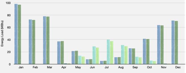
Conventional Roof Cooling Load Green roof Cooling Load Green roof Heating Load Green roof Heating Load
