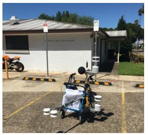
West Sydney. The incident solar radiation reflection ratio (albedo) of these carparks was also measured. Asphalt pavements, for instant, absorb 90% of incoming solar radiation, then released as heat by convection.
