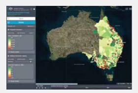
The project uses the Dynamic Avoidable Network Cost Evaluation (DANCE) model developed by ISF as part of the Intelligent Grid research program. ISF has previously applied the DANCE model for mapping Decentralised Energy for Victoria and for rural areas of the NEM suitable for concentrating solar power.
