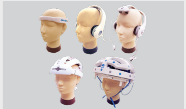
EEG headsets have range of sensors to detect electrical activity in different areas of the brain for augmented human performance Photo: US Army Research Lab
